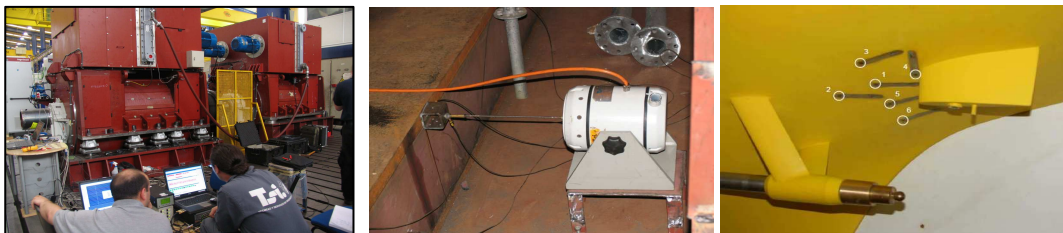
Figure 7.- FAT, Inertance and Model Tests, developed for the Design of the “ Ramón Margalef ”.-
